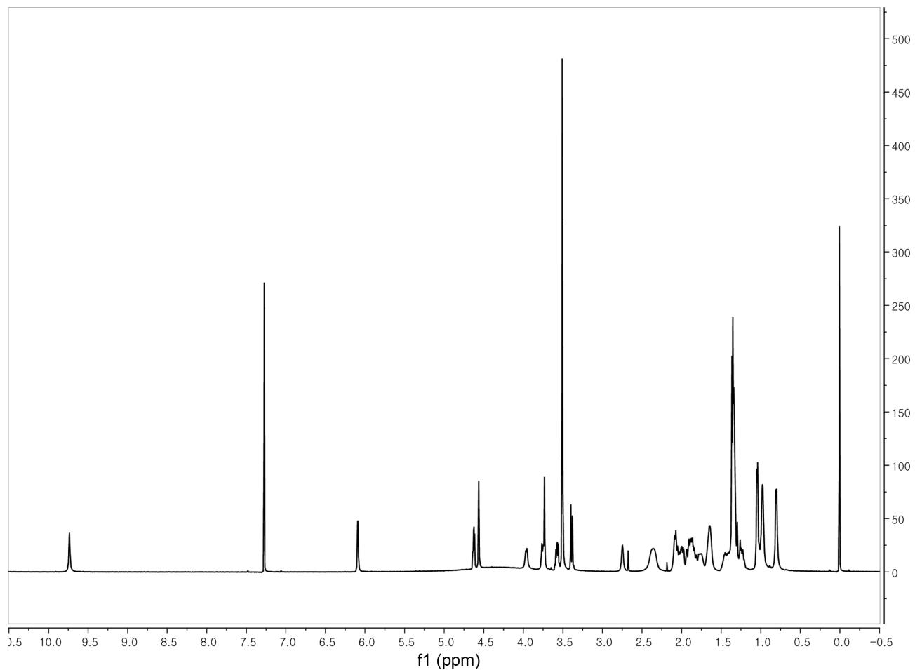
**Supplementary Fig. 1.**  $^1\text{H}$  NMR spectrum (500 MHz) of morinifungin in  $\text{CDCl}_3$ . NMR, nuclear magnetic resonance.
